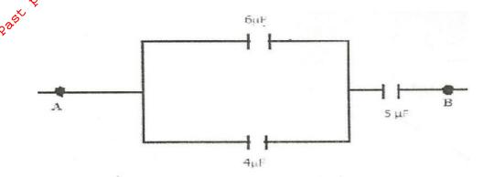
Determine the p.d across the  $5\mu F$  capacitor given that the total charge stored in the capacitors is 0.0000052~C. (3 marks)
