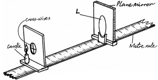
Describe how the set-up may be used to determine the focal length, f, of the lens. (4 marks)
