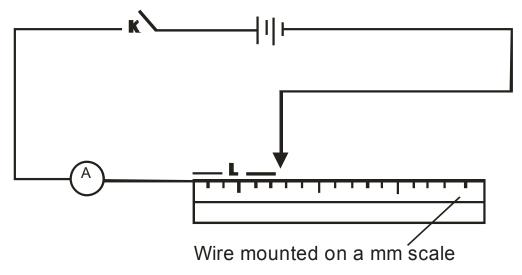
c) Adjust the length L of the wire to 0.1m, close the switch k, and read the value of current and record in the table below.
