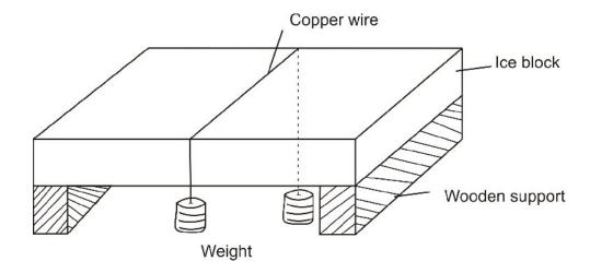
It is observed that the wire gradually cuts its way through the ice block, but leaves it as one piece.
