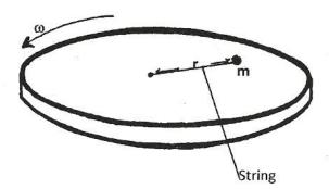
The tension T, on the string was measured for various values of angular velocity,  $\omega$ . The distance rfrom the centre was maintained at 30cm. The results are as shown below :
