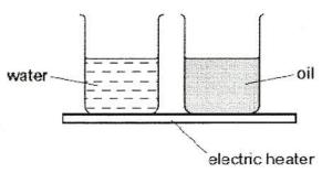
The temperature of the water and the temperature of the oil increase constantly. The rise in temperature of the oil is much greater than that of the water. (1mk)
