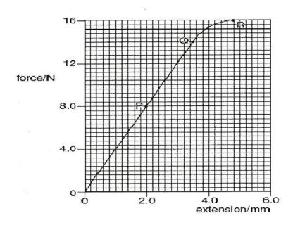
The part OP of the graph shows the springs stretching according to the expression F = kx.
