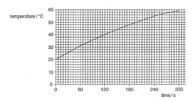
The piece of metal is heated in boiling water until it has reached the temperature of the water. It is then transferred rapidly to some water in a well-insulated cup. A very sensitive thermometer is used to measure the initial and final temperatures of the water in the cup.
