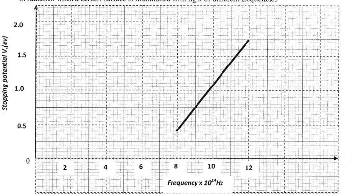
From the graph determine the work function of the metal surface. ( $h=6.63 \times 10^{-34} Js$ ) (2mks
