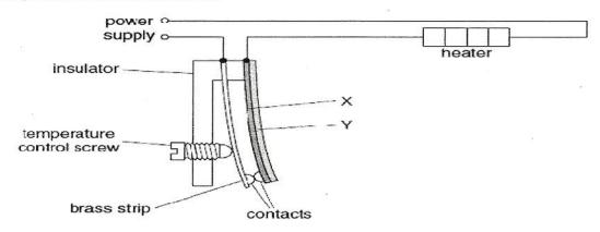
X and Y are strips of two different metals, joined together along their length. Together they are called a bimetallic strip. X expands more than Y for the same temperature rise. The temperature rises and the bimetallic strip bends. State
