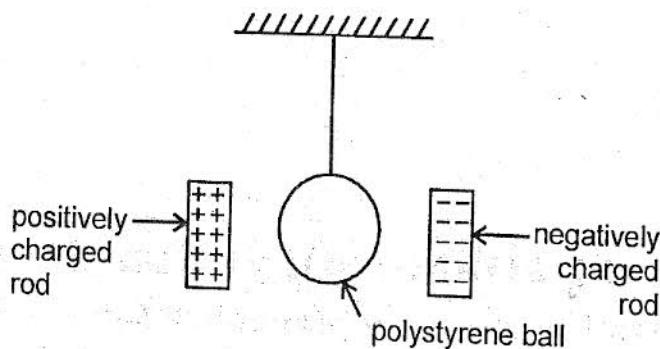
The ball is found to swing between the two rods as it touches one of them at a time. Explain the cause of this behavior of the ball between the rods.
