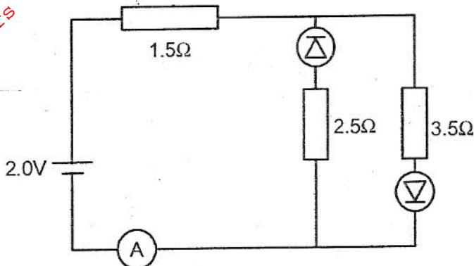
Determine the ammeter reading given that the cell has an e.m.f of 2.0V.
