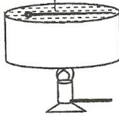
Steel needle floating on water surface
