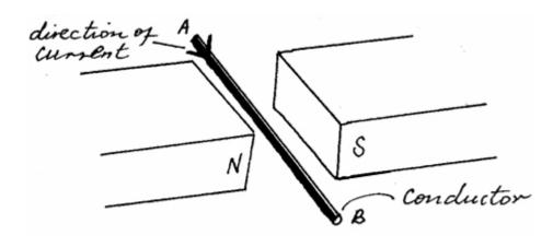
(a) Indicate the direction of force F acting on the conductor.
