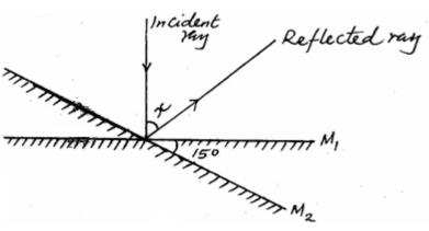
Determine the angle between the reflection ray and the incident ray.
