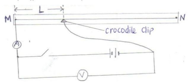
ii) Remove the crocodile clip from the resistance wire MN and close the switch. Record the voltmeter reading.
