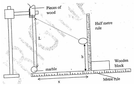
(III) Adjust the clamp so that the marble is next to the end of the metre rule as shown above.
