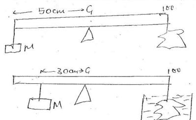
The solid and the mass m are the same throughout the experiment. Calculate the relative density of the solid.
