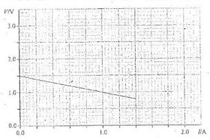
i) Show how the relationship V = E - Ir can be used with his graph to determine the e.m.fE of the cell. State its value.
