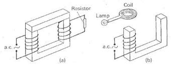
i) If the primary coil is connected to a 240 V a.c mains supply what will be the secondary voltage.
