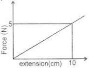
How much work is done in stretching this spring by 8cm.
