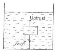
c) A piece of wood of mass 12g is kept under water by means of a string as shown the figure above. Its volume is 30cm<sup>3</sup>. a Attemet
