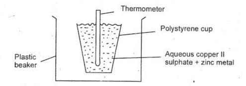
1.0g of zinc powder was added to 50cm³ of 0.2N Copper II Sulphate solution and the mixture steamed gently, the temperature rose from 21°C to 28°C.
