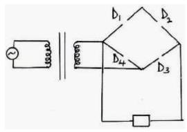
(c) Explain why a bridge rectifier circuit is better than a single diode rectifier circuit. (1mk)
