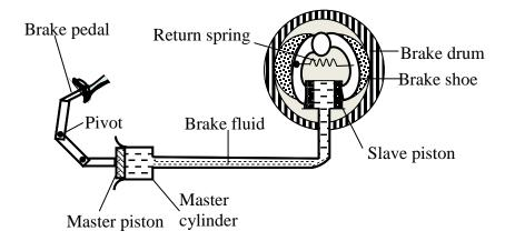
The brake drum rotates with the wheel of the car.
