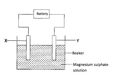
During the electrolysis, hydrogen gas was formed at electrode Y. i) the anode. Give a reason for your answer. identify (2marks)
