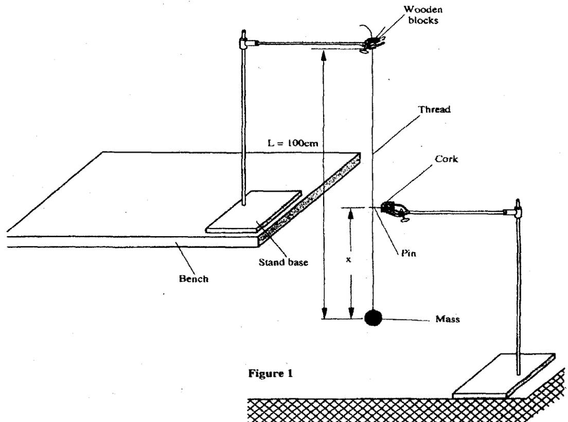
The thread tied to the mass should be held firmly between the two blocks of wood and clamped to the upper end of the stand so that the mass hangs freely. The distance  $L$  between the point of support and the centre of the mass is 100 cm. Ensure that  $L$  remains constant throughout the experiment.
