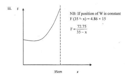
iv). As x increase / anticlockwise moments reduces/ moments to the left reduces/ distance between F and pivot reduces F has to increase to maintain equilibrium.
