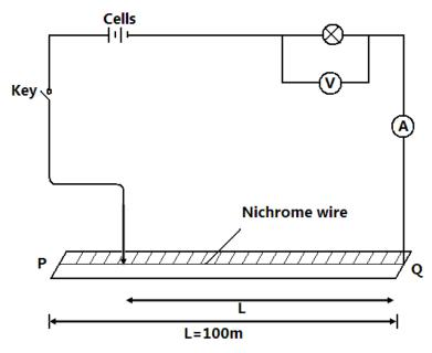
ii) With the crocodile clip at p, take the voltmeter reading and ammeter reading. Record v and 1 repeat the readings for L=80, 60, 40, 20 and 0cm respectively and complete the table below.
