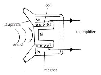
(i) Explain how a velocity current is induced in the coil when the diaphram vibrates (3mks)
