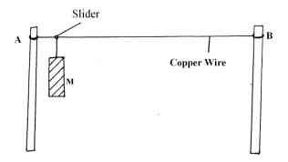
The copper wire is then heated for sometime, State and explain what is likely to be observed on the position of the mass. (2mks)
