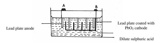
(i) The electrolyte used in the cell is dilute sulphuric acid, why is dilute hydrochloric acid not used. (1 mk)
