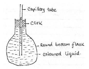
State what will be observed when the above apparatus is placed in cold water.
