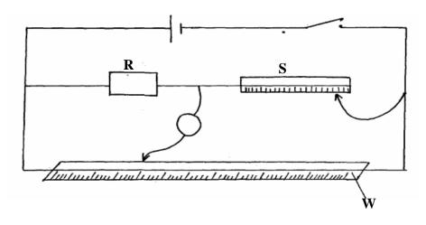
(c) Close the switch, and use the jockey to touch one end of the wire W, and then the other end. The deflections on the galvanometer should be in opposite directions, if not check the circuit. Adjust the positions of the jockey along the wire W until there is no deflection in the galvanometer. Record the value of x and y.
