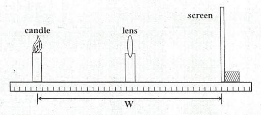
Adjust the position of the lens to obtain a sharp enlarged image of the candle
