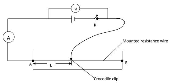
Place the crocodile clip/jockey on the wire AB starting with  $L=20\ cm$ . Close the switch K. Record the terminal p.d., V and corresponding current I. Repeat for other values of L shown and complete the table.
