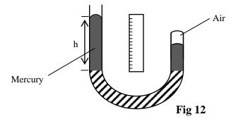
By raising the open end of the tube, the student measured the corresponding values of the length L, of the air column and the excess pressure.
