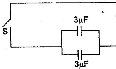
Determine the charge stored in the combined capacitors when the switch (S) is closed. (3 marks)
