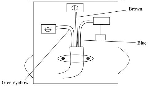
a) i) Identify two mistakes in this wiring.
