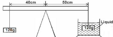
By displacement method, the immersed object is found to occupy 13.5cm<sup>3</sup>. Determine the density of the liquid in SI units. marks)
