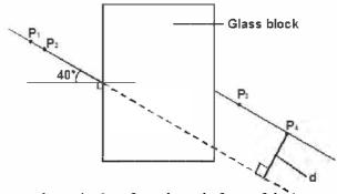
ii) Draw normal at point 2cm from the end of one of the longer side of the block outline. Draw a line at an angle of  $\Box$  = from the normal. Stick two pins  $p_1$  and  $p_2$  vertically on this line.
