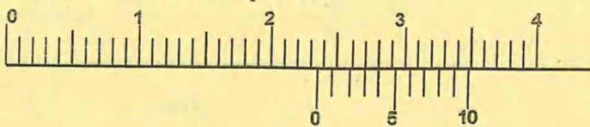
Determine the actual reading of the scale if the instrument has zero error of 0.02cm (2 marks)
