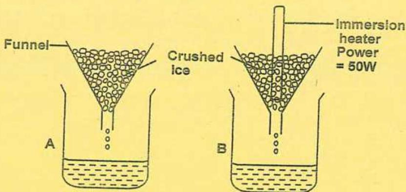
The mass of melted ice on each funnel is measured after 12 minutes.
