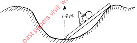
i) Determine the velocity ratio of the arrangement
