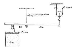
The area of the piston is  $10\text{cm}^2$  and the volume of the gas is  $20\text{cm}^3$ . The weight of the pulley, the beam and the frictional forces at the movable parts are taken to be zero. If the beam is in equilibrium,
