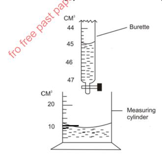
2cm³ of water was added in the cylinder from a burette. Record in the spaces provided below the new readings indicated in each vessel(2mks)
