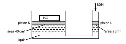
(i) Find the pressure at piston L in N/m<sup>2</sup>.(1mk)
