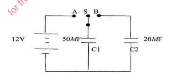
(i) The switch S is first placed at position A, so that the capacitor C, is connected to the 12V dc supply. Calculate the charge stored in the capacitor. (3marks)
