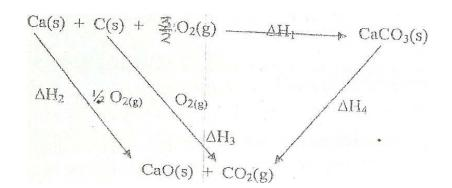
Given:  $\Delta H_1 = -1207 \text{ kj/mol}$ ,  $\Delta H_2 = -635 \text{kj/mol}$ ,  $\Delta H_3 = -394 \text{kJ/mol}$
