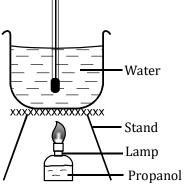
During the experiment the data given below was recorded. Volume of water  $= 100 \text{cm}^{3}$ Final temperature of water  $= 43.5^{\circ}C$ Initial temperatures of water  $= 20.5^{\circ}C$ Mass of propanol + lamp before burning = 126.5gMass of propanol + lamp after burning = 124.7g
