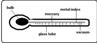
It's used to measure the highest temperature reached in a day. It uses mercury.
