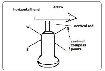
Wind direction is determined using wind vane.
