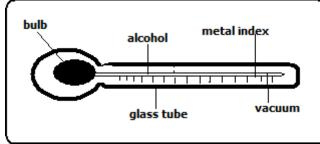
It's used to record the lowest temperature reached in a day.
