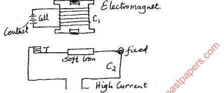
b) When switch is closed electromagnet attracts soft iron. This causes T to close and so circuit 2 is put on.
