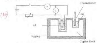
I) Other than temperature and current, state two measurements that should be taken in the experiment to determine the specific heat capacity of the block. (2marks)
