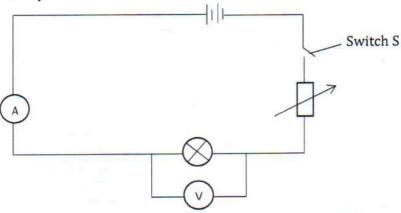
Close the switch S and adjust the potentiometer P till the bulb lights brightest. Record the ammeter and voltmeter reading.
